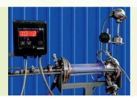
This category of burner devices is characterized by a great durability of work under load (up to 5,000 ... 7,000 hours without stopping work.) Due to the low complexity of the design, maintenance and repair do not require highly qualified personnel.
